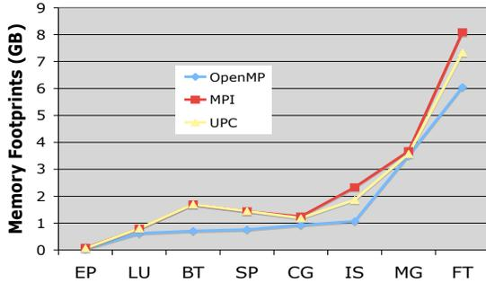
Fig. 2. The memory footprints of NPB3.3 applications for MPI, OpenMP, and UPC for four-core runs.
