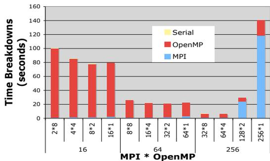
Fig. 7. The BT-MZ Time Breakdown on Hopper.
