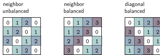
Fig. 2 Combinations of mapping properties. Numbers in blocks indicate the unit rank owning the block.
